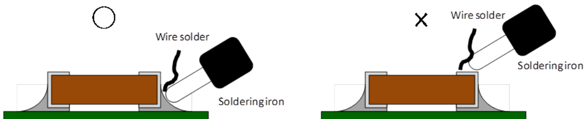
Fig 3 Correct handling method of soldering iron
